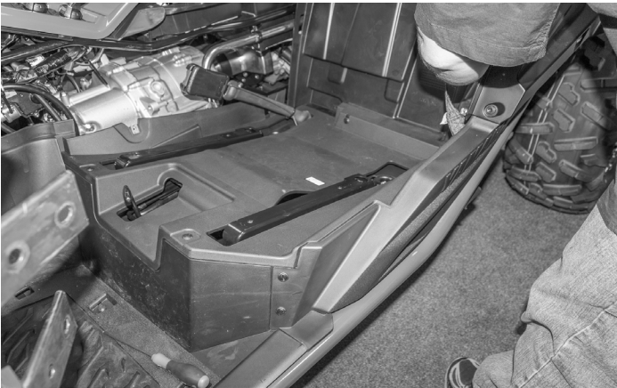
Reinstall the other under seat panel and exterior panel.
