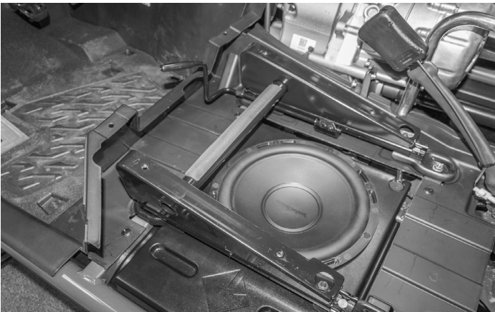
Bolt in the seat slider and apply foam to the slider tube to prevent rattles.
