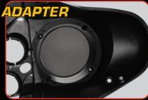
Align adapter with factory screw holes and attach with supplied screws. Be sure gasket is properly seated between grille and adapter.
