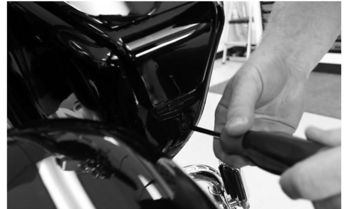
After the screws are removed, use your socket or ratcheting wrench to unbolt the turn signal brackets.
