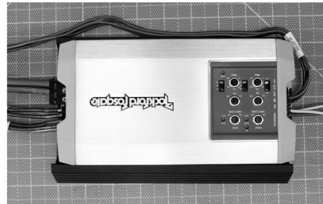
Note: Refer to your amplifier owner's manual for additional wiring and setup information. Be careful when plugging in the harnesses to the appropriate socket. The 4-pin Molex plugs for the Input / Output Harnesses fit in both sides of the amplifier.
