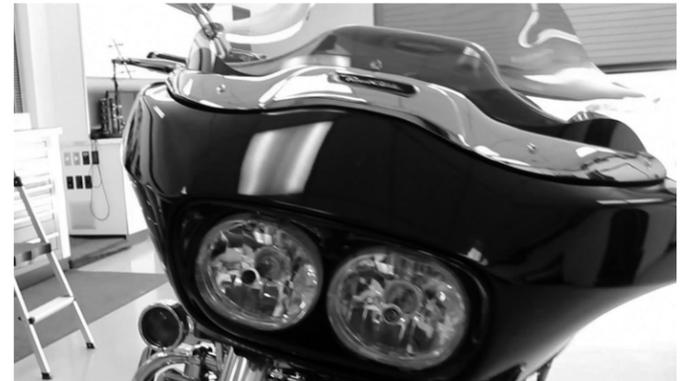
Leaving the windshield in place, remove the six inner fairing screws.
