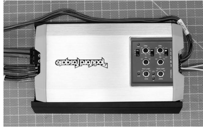
Note: Refer to your amplifier's owner manual for additional wiring and setup information. Be careful when plugging in the harnesses to the appropriate socket. The 4-pin Molex plugs for the Input / Output Harnesses fit in both sides of the amplifier.
