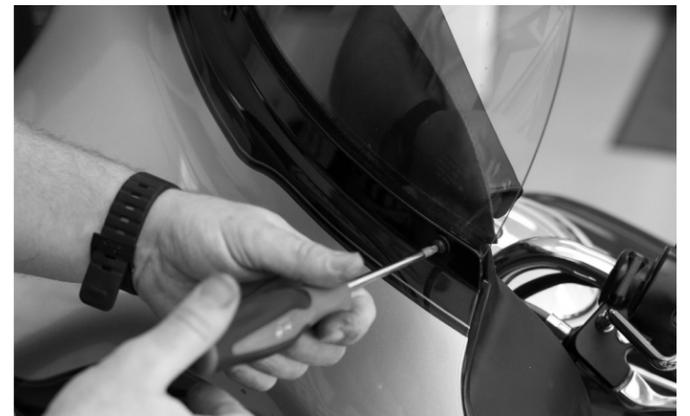
Once you have the windshield set aside, remove the remaining screws on the inside of the fairing. This will allow you to remove the front fairing.
