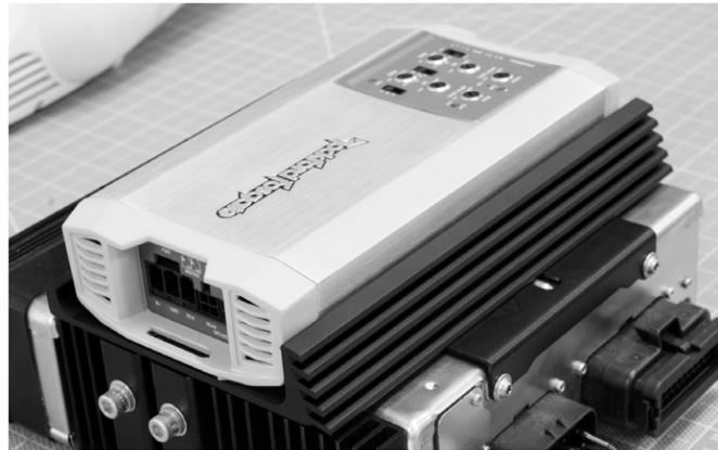
Once the amplifier is mounted, you can now begin plugging in the wiring harness in their appropriate sockets.
