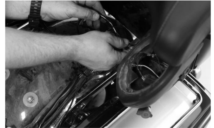
Unplug the factory speaker wires from the speaker and plug them directly in to the Rear Speaker Input / Output Harness. These are labeled clutch and brake side.
