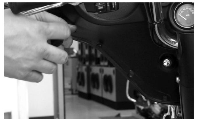
You will need to disconnect the harness from the headlight to completely take the fairing off of the motorcycle.
