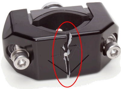
Top Fracture Caused by Over Tightening
