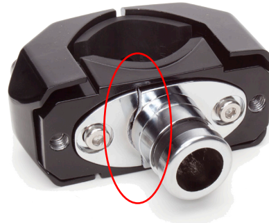
Bottom Fracture Caused by Over Tightening
