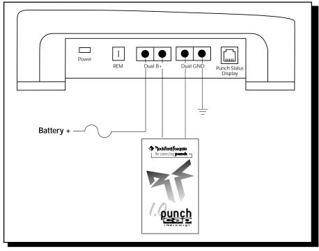
• Recommended capacitance is 1 farad per 1000 watts
