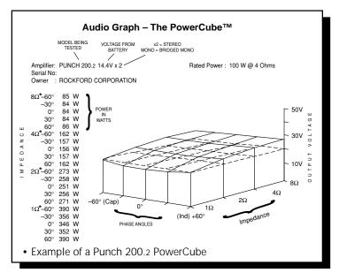
Therefore, a perfect amplifier will be able to maintain the same output voltage regardless of load characteristics and will not alter the signal it is reproducing. A perfect amplifier when measured by the Audio Graph PowerCube would present data that forms a perfect cube. Unfortunately, amplifiers are not perfect. The laws of physics generally prevent it. A great amplifier is about the best one can hope to attain.
