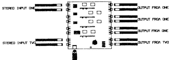
6. TWO INPUTS - ONE INPUT FEEDING TWO OUTPUTS
