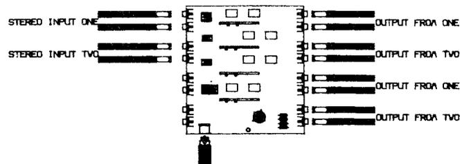
5. TWO INPUTS - ONE INPUT FEEDING THREE OUTPUTS
