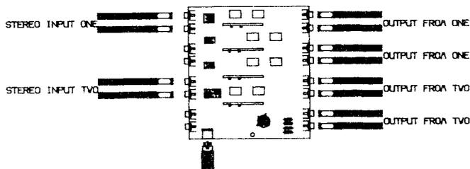
7. THREE INPUTS - ONE INPUT FEEDING ONE OUTPUT
