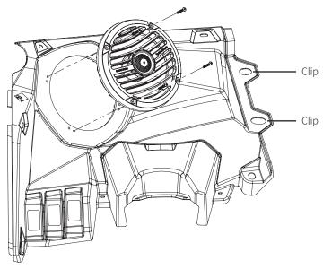
Remove the remaining screws that secure the driver / passenger dash panel.
